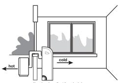
Hang "condenser" out through window (supplied with hanging straps and hooks) or drill hole through wall.
